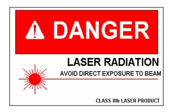
➡ Class 4 laser warning is always DANGER followed by the wording explaining how to protect oneself and a description of the specific laser that is in use, for example: "INVISIBLE LASER RADIATION AVOID EYE OR SKIN EXPOSURE TO DIRECT OR SCATTERED RADIATION"
